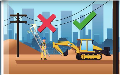
7 Do not approach plant or equipment that might be in contact with the power lines
