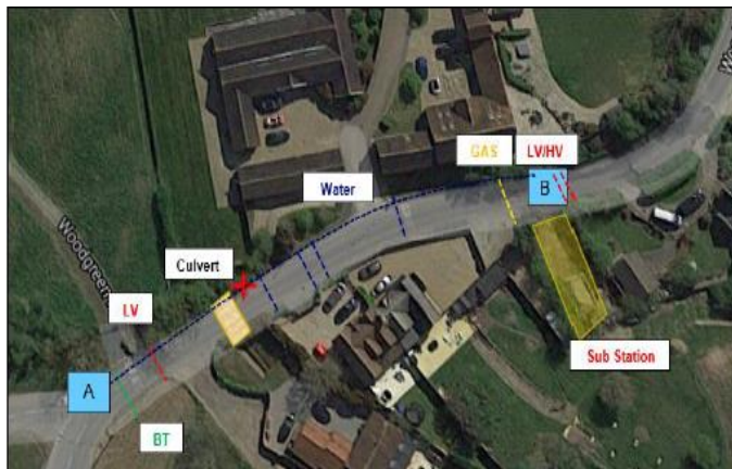
Overlay of the utility crossing points on the directional drilling path exposed by the site team
