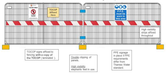
Alternatives to HERAS fencing such as hoarding are permitted but the TOCOP area must be clearly delineated from any areas not covered under the TOCOP.
