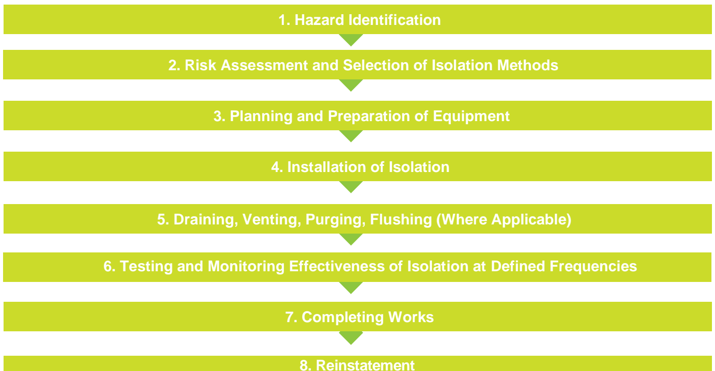
Fig 1. Safe isolation procedure
