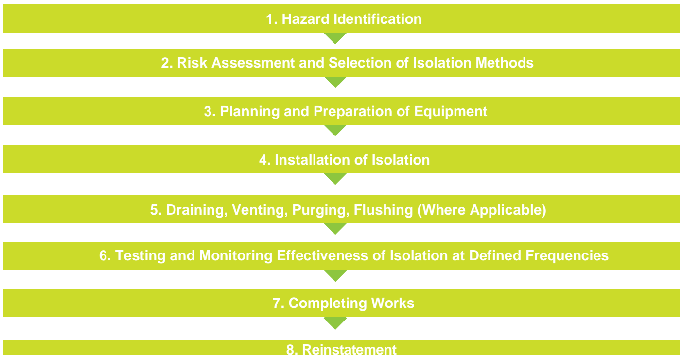
Fig 1. Safe isolation procedure
